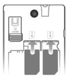
Remove the battery cover and the battery, then insert the SIM cards into the corresponding slots with the gold-coloured contacts facing down.
